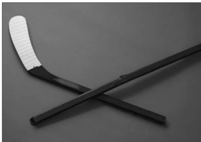
Fig. 1. Composite hockey stick that penetrated left axilla of patient. Stick is fractured in 2 places, rendering 3 fragments.
