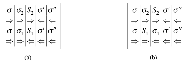
Figure 1. Space–time history for a right move (\sigma_1, S_1) \rightarrow (\sigma_2, (S_2, RIGHT)) .
