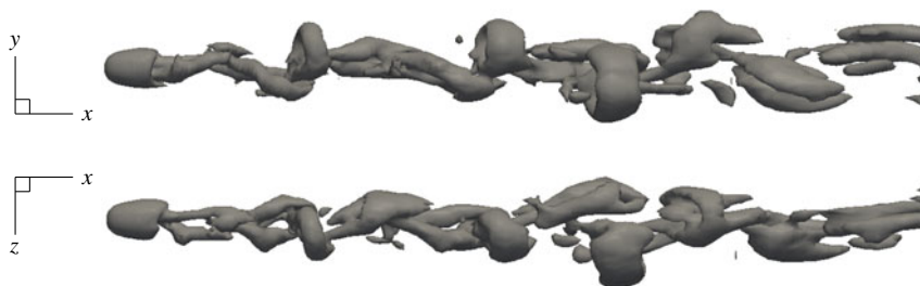
FIGURE 26. Instantaneous wake structure of a stationary sphere at Re = 800 .
