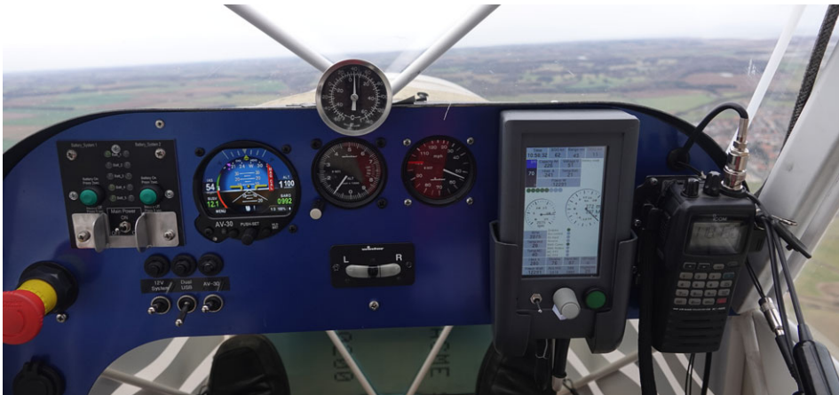
Figure 3. Sherwood eKub's instrument panel. Left to right showing eSTOP emergency powertrain control, battery management panel, AV30 mini-EFIS, altimeter, cockpit thermometer (above), turn co-ordinator (below), airspeed indicator, ADI unit, VHF radio.
