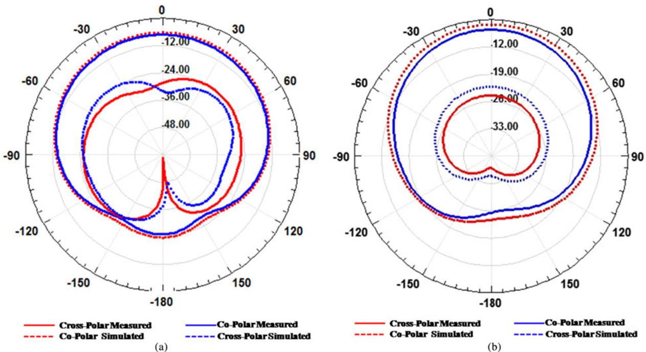
Fig. 15. Simulated and measured co-polar and cross-polar radiation pattern of Ant<sub>2</sub> (with trapezoidal shaped DGS) at frequency 1.85 GHz, (a) E-plane, (b) H-plane.
