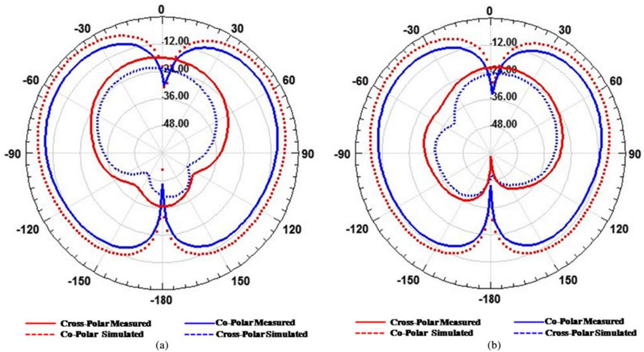
Fig. 14. Simulated and measured co-polar and cross-polar radiation pattern of Ant<sub>1</sub> (without DGS) at frequency 4.9 GHz, (a) E-plane, (b) H-plane.
