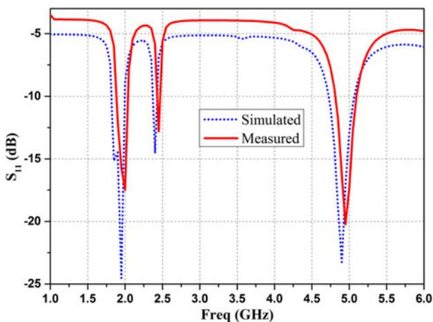
Fig. 4. Simulated and measured  $S_{11}$  variations with frequency of Ant<sub>1</sub>.
