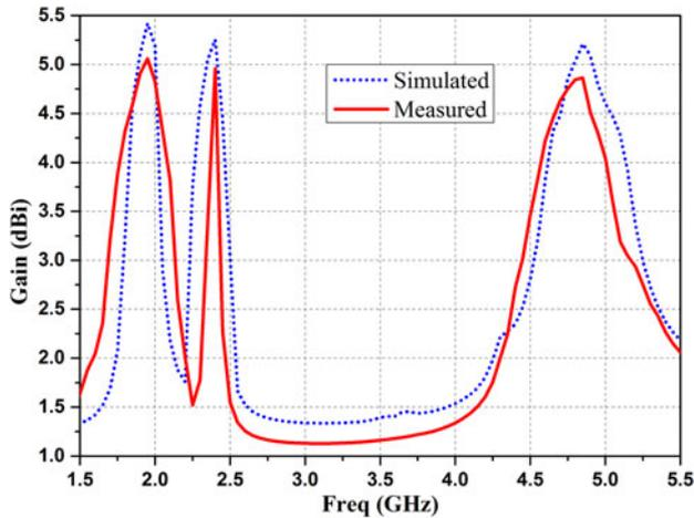
Fig. 12. Simulated and measured Antenna Gain variations with frequency of Ant3.
