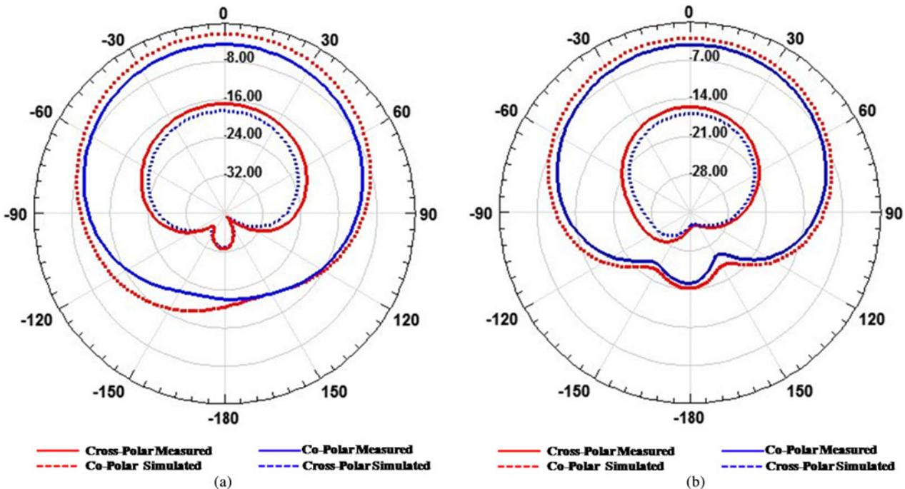
Fig. 13. Simulated and measured co-polar and cross-polar radiation pattern of Ant1 (without DGS) at frequency 1.95 GHz, (a) E-plane, (b) H-plane.
