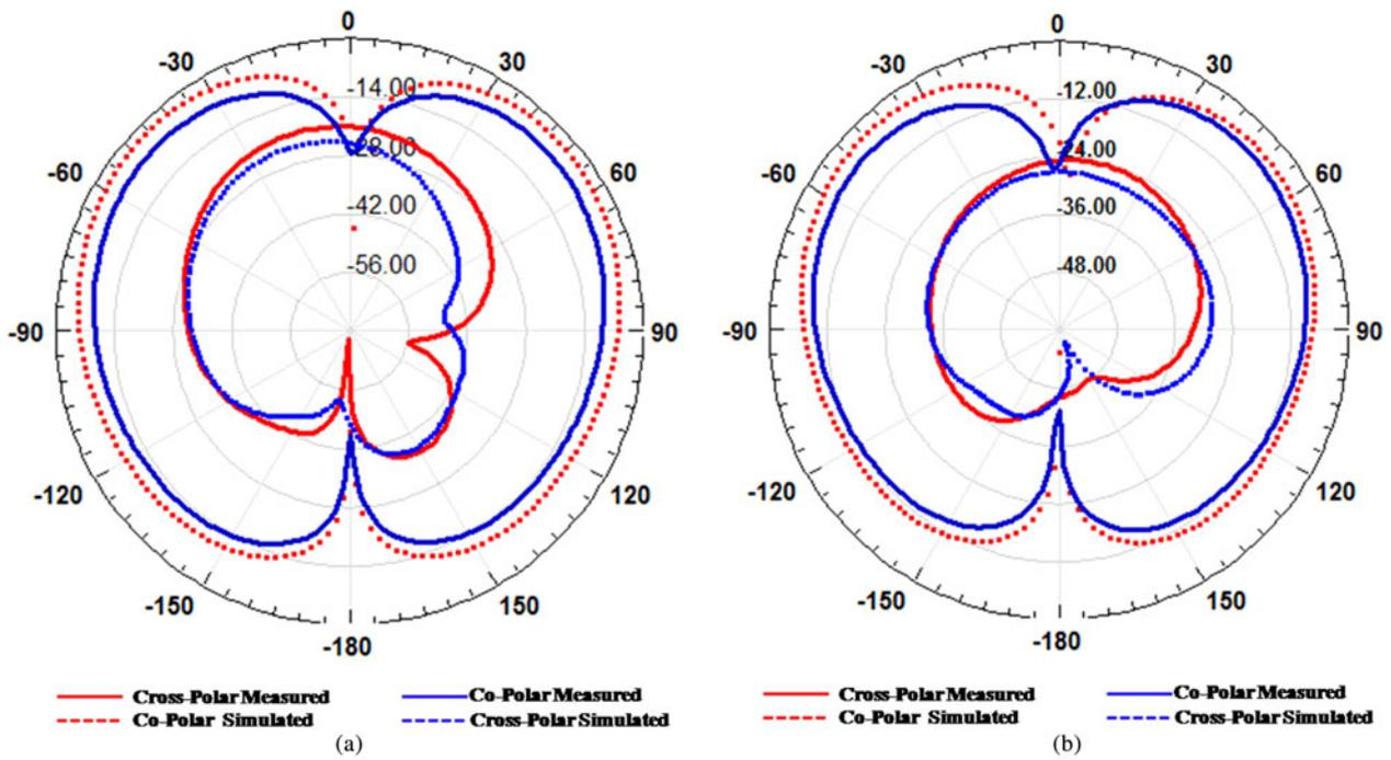
Fig. 16. Simulated and measured co-polar and cross-polar radiation pattern of Ant2 (with trapezoidal shaped DGS) at frequency 4.85 GHz, (a) E-plane, (b) H-plane.
