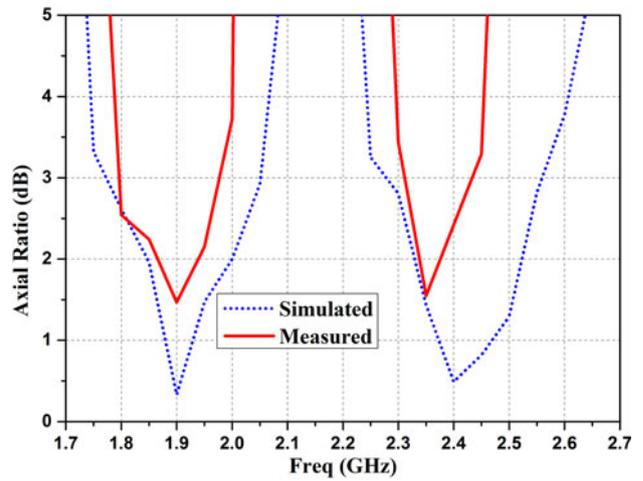
Fig. 9. Simulated and measured Axial Ratio variations with frequency of Ant3 (with DGS).
