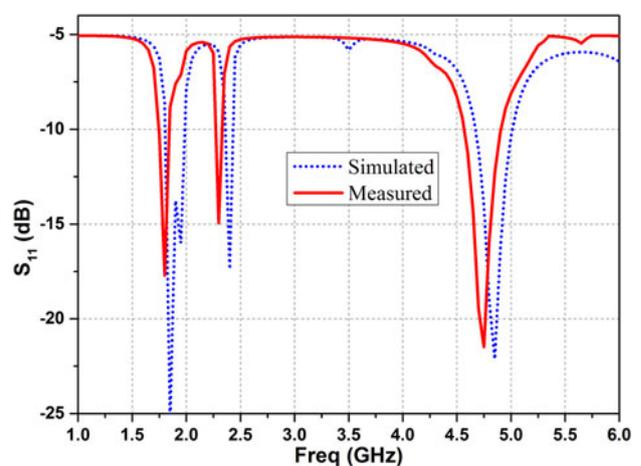
Fig. 5. Simulated and measured  $S_{11}$  variations with frequency of Ant<sub>2</sub>.
