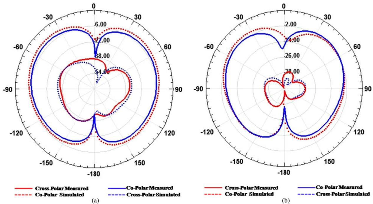
Fig. 18. Simulated and measured co-polar and cross-polar radiation pattern of Ant3 (with DGS) at frequency 4.85 GHz, (a) E-plane, (b) H-plane.
