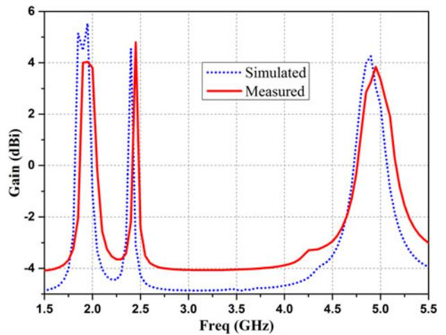
Fig. 10. Simulated and measured Antenna Gain variations with frequency of Ant1.
