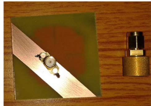
Fig. 2. Structure of the proposed antenna Ant2 (with trapezoidal shaped DGS); (a) schematic, (b) top view of fabricated Ant2, (c) bottom view of fabricated Ant2.
