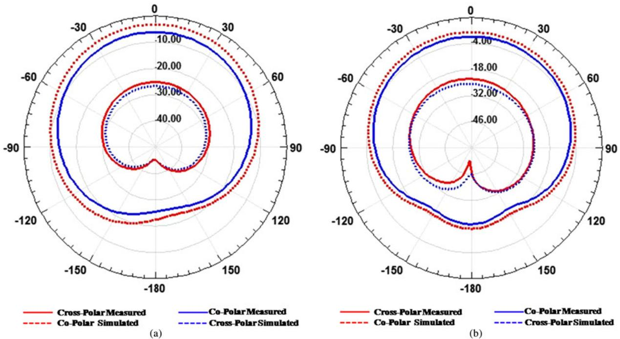
Fig. 17. Simulated and measured co-polar and cross-polar radiation pattern of Ant3 (with DGS) at frequency 1.95 GHz, (a) E-plane, (b) H-plane.
