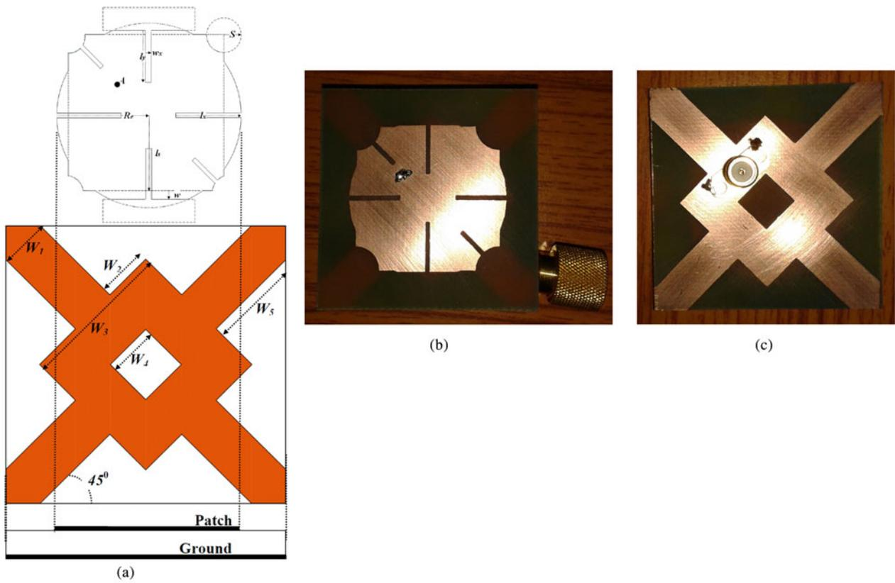
Fig. 3. Structure of the proposed antenna Ant<sub>3</sub> (with DGS); (a) schematic, (b) top view of fabricated Ant<sub>3</sub>, (c) bottom view of fabricated Ant<sub>3</sub>.
