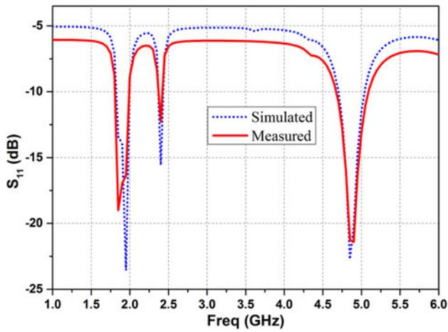
Fig. 6. Simulated and measured  $S_{11}$  variations with frequency of Ant3.
