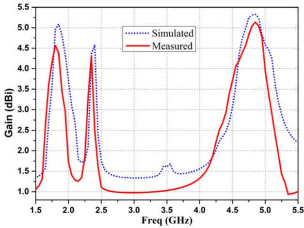
Fig. 11. Simulated and measured Antenna Gain variations with frequency of Ant2.
