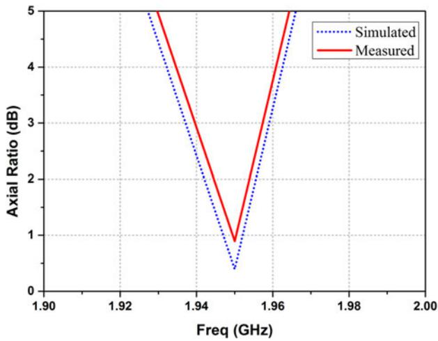
Fig. 7. Simulated and measured Axial Ratio variations with frequency of Ant1 (without DGS).
