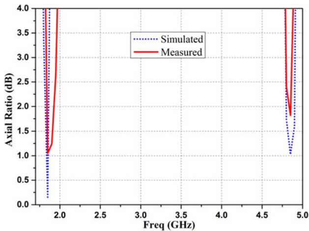
Fig. 8. Simulated and measured Axial Ratio variations with frequency of Ant2 (with trapezoidal shaped DGS).
