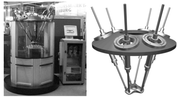
Fig. 3. Case study: Hexapod PaLiDA. Left: presentation in the Hannover industrial fair, 2001. Right: CAD model.
