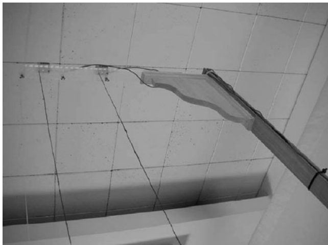
Figure 6b. A detail of the upper part of the pendulum apparatus. The horizontal bar is made of Plexiglas. The load cells used for measurements of the tension in the strings can be seen on the Plexiglas bar (see Palmieri, Reenacting Galileo's Experiments , Appendix 2).
