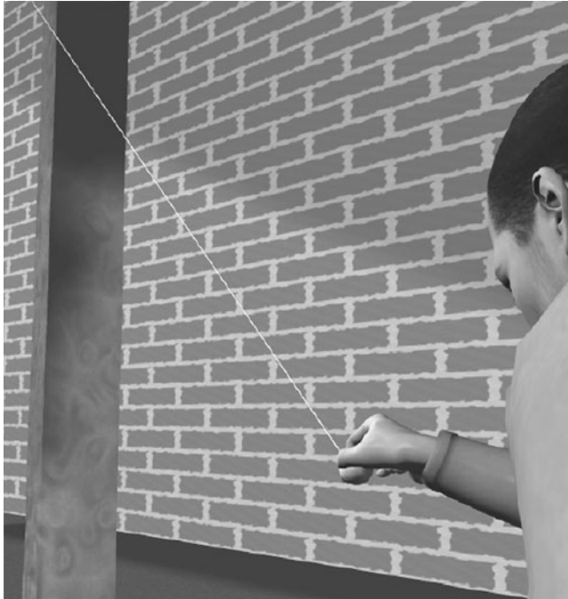
Figure 3b. The operator ‘takes aim’, as it were, trying to position the hand which grabs the bob in such a way that the motion of the pendulum remains as much as possible in a non-rotating plane. Since the pendulum is attached to a string, its oscillation plane has a tendency to deviate uncontrollably. Yet to a certain extent the operator learns how to sense and prevent this effect before releasing the bob.
