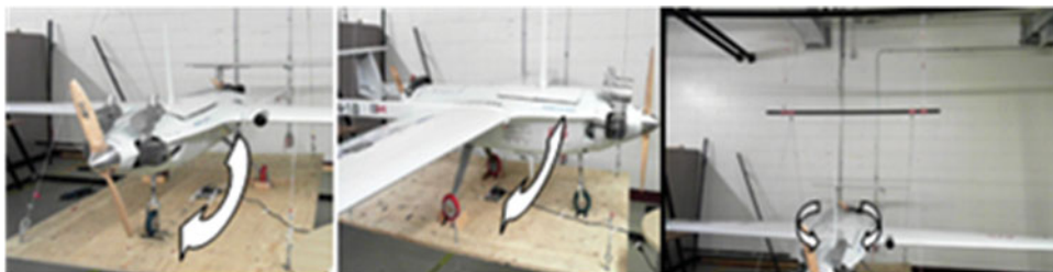
Figure 27. (Colour online) Swing test about the Y, X and Z axes.
