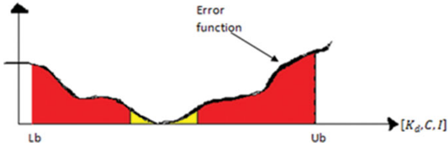
Figure 20. (Colour online) The Error Function variation with three parameters ( K_d , C , I ). Search field of 'ga' (in red) and 'fminsearch' (in yellow) functions.
