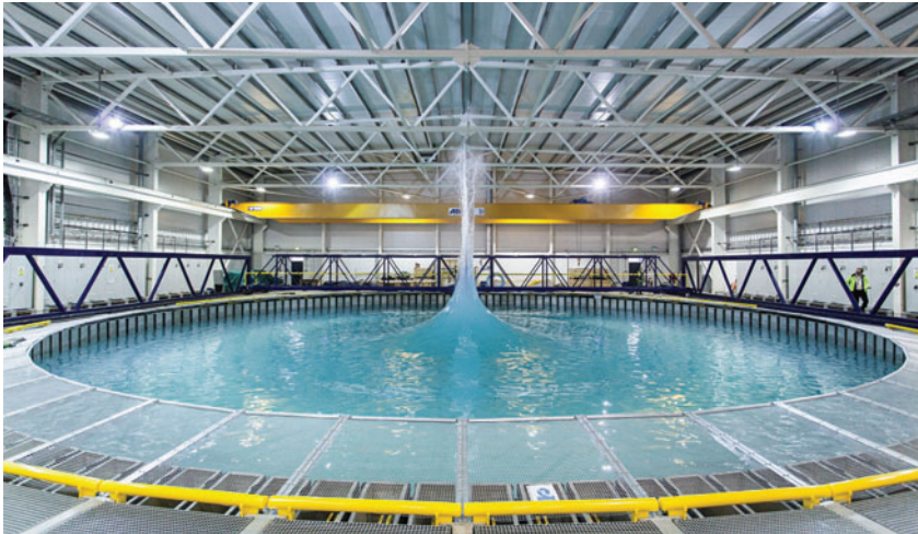
Figure 1. Image of the ‘spike wave’ created in the FloWave circular wave tank.
