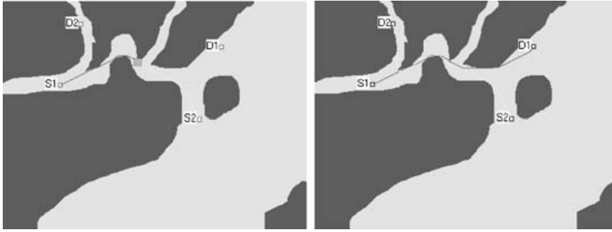
Figure 7. Illustration of the shortest path algorithm with collision avoidance scheme for two ships.
