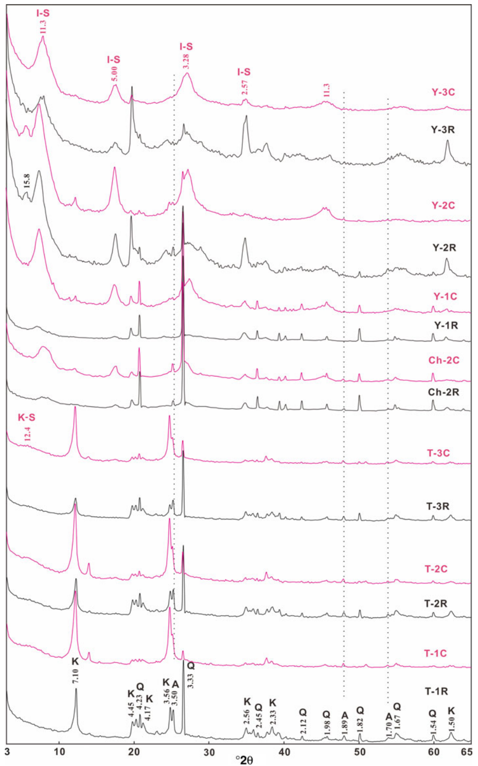
Fig. 2. XRD traces of the clay fraction and remnant. I-S = mixed-layer illite-smectite; K = kaolinite; Q = quartz; F = feldspar; A = anatase; I = illite; T-1C, T-2C, T-3C, Ch-2C, Y-1C, Y-2C, Y-3C = clay fractions of Tucheng, Chahe, and Yanlou sections, and T-1R, T-2R, T-3R, Ch-2R, Y-1R, Y-2R and Y-3R are the remnant counterparts.
