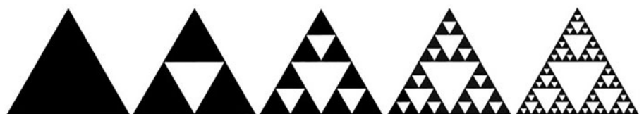
Fig. 3. Sierpinski gasket geometry till 4 th iteration (0 th , 1 st , 2 nd , 3 rd , and 4 th iteration) [2].
