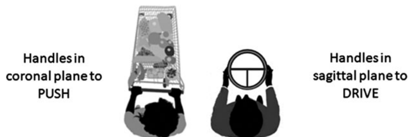
Fig. 6. Handle directions and their functions: push or drive.
