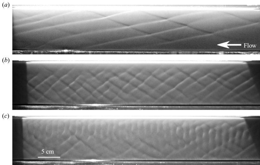
FIGURE 1. Various bedforms observed on the granular bed of a laminar flume (Devauchelle et al. 2009). The flow is from right to left. The pattern, observed through the water surface, is enhanced by skimming light. The angle and wavelength of the rhomboid pattern varies with the experimental parameters ((a) and (b)). Under certain conditions, ripples can coexist with a rhomboid pattern (c). The width of the flume is 10 cm. (a) Large rhomboid pattern ( Fr = 1.76 , S = 0.03 , Bo = 1.31 and Sh = 0.616 ). (b) Small rhomboid pattern ( Fr = 0.95 , S = 0.015 , Bo = 3.25 and Sh = 0.485 ). (c) Rhomboid pattern mixed with ripples ( Fr = 1.01 , S = 0.015 , Bo = 3.50 and Sh = 0.504 ). The definitions of the parameters are provided in § 3.2.
