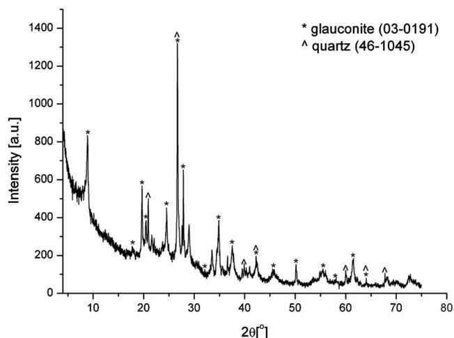
Figure 6. XRD pattern for green fragments of Ruthenian-Byzantine frescoes from St. Mary's Chapel of Wawel Cathedral after removal of calcite.
