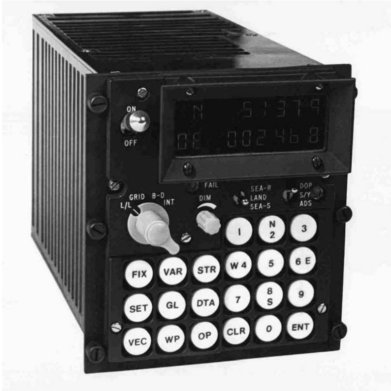
Figure 3. TANS (Tactical Air Navigation System) computer 9447D used with the Type 71.
