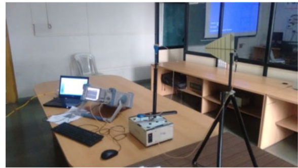
Fig. 9. Set-up to measure the radiation characteristics of the proposed design.
