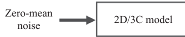
FIGURE 3. The approximation for illustrating the 2D/3C model’s lack of robustness. The zero-mean noise is used as an approximation for the modelling errors and uncertainty. The noise acts as an additive ‘uncertainty’ at each time step.
