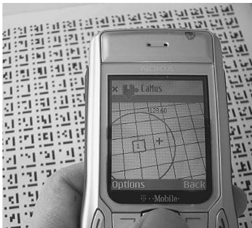
Figure 2. CaMus uses the built-in camera over a two-dimensional marker sheet to allow motion in a virtual space.
