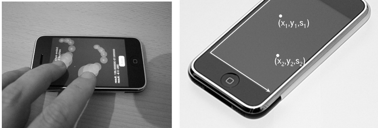
Figure 6. (Left) Fendrix is a multi-sensor instrument implemented on the iPhone. Multiple fingers can trigger multiple continuously controlled voices. (Right) Coordinate space of the iPhone multitouch interface.
