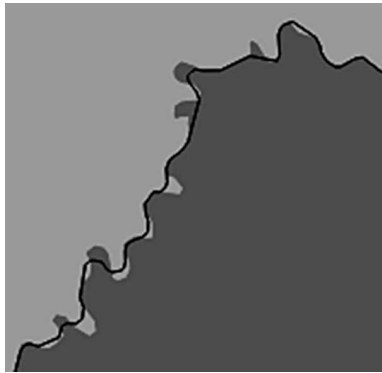
Figure 7. Misaligned boundaries. Different sources of data place state and district boundaries in different places. The border shown here lies between Maryland 06 and West Virginia 01. The “true boundary” is drawn from data at 1:500,000 resolution and is shown by the transition between solid colors, while the black line shows the same boundary using 1:5,000,000 data. Differing data resolutions is only one instance in which a mismatch might occur: Shifts in data (as from projections), differing collection procedures, or deliberate manipulation are all possible as well.
