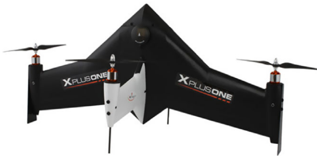
Figure 14. X Plus One, a differential thrust transitioning tail-sitter hybrid VTOL UAV. Image adopted from reference [101], with permission.
