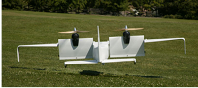
Figure 6. AT-10 Responder aircraft, a tilt-wing hybrid VTOL UAV, during vertical takeoff. Image adopted from Acuity Technologies [38], with permission.
