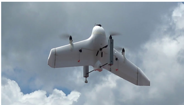
Figure 16. Quad-rotor Tail-sitter hybrid VTOL UAV in hover flight mode. Image adopted from reference [112], with permission.
