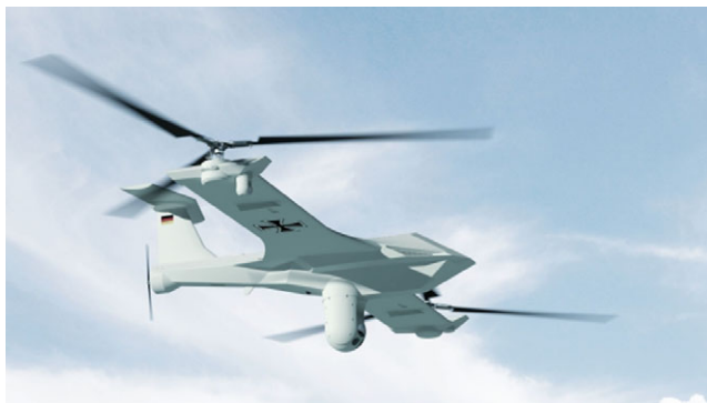
Figure 9. TU-150 aircraft, a bi-rotor dual system hybrid VTOL UAV. Image adopted from reference [51], with permission.
