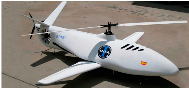
Figure 8. Helicopter ADaptive Aircraft (HADA), a dual system hybrid VTOL UAV. Image adopted from reference [58], with permission.
