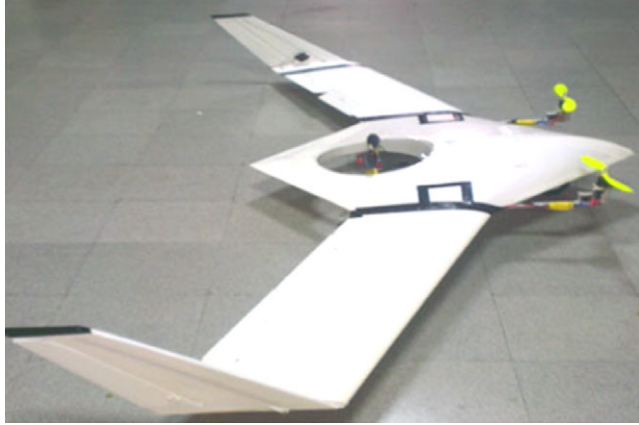
Figure 3. TURAC aircraft, a tilt-rotor hybrid VTOL UAV with two forward tilting rotors and one ducted coaxial fan. Image is adopted from reference [7], with permission.
