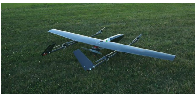
Figure 17. SuperVolvo hybrid VTOL UAV, being developed by GE Aviation, USA. Image adopted from reference [105], with permission.
