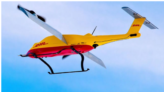
Figure 7. DHL Parcelcopter 3.0, a tilt-wing hybrid VTOL UAV with single wing configuration, shown in the transition phase of flight. Image adopted from DHL [39, 40], with permission.
