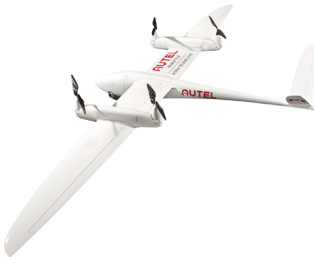
Figure 2. Kestrel aircraft, a quad-tilt-rotor hybrid VTOL UAV. Image is adopted from Autel Robotics [13], with permission.
