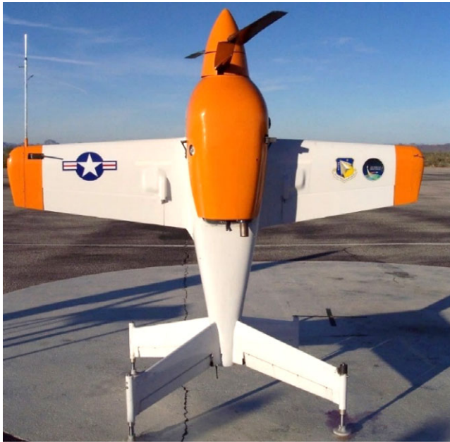
Figure 10. SkyTote aircraft, a mono thrust transitioning, tail-sitter hybrid VTOL UAV. Image adopted from reference [66], with permission.
