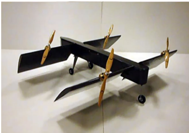
Figure 5. SUAVI aircraft, a tilt-wing hybrid VTOL UAV with tandem wing configuration. Positioning of wings shown in the figure corresponds to the transition phase of flight. Image adopted from reference [45], with permission.
