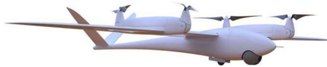
Figure 4. Quantum Tron a quad-tilt-rotor hybrid VTOL UAV. Image is adopted from reference [15] with permission.
