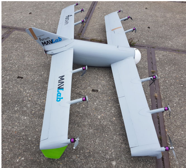
Figure 15. NederDrone2 aircraft, a hybrid VTOL UAV being manufactured by Delft University of Technology. Image adopted from reference [104], with permission.
