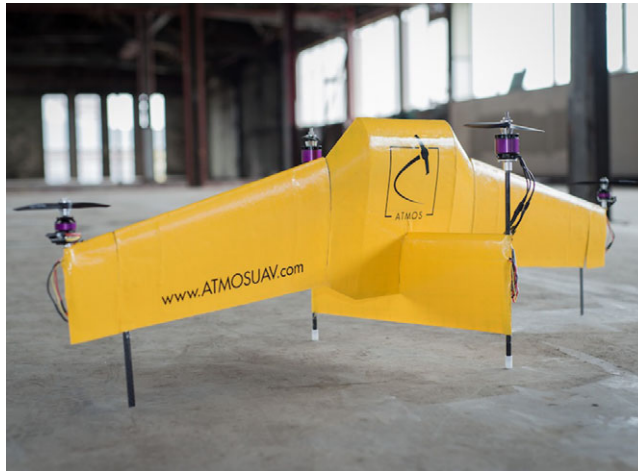
Figure 13. ATMOS UAV, a differential thrust transitioning tail-sitter hybrid VTOL UAV. Image adopted from reference [102], with permission.
