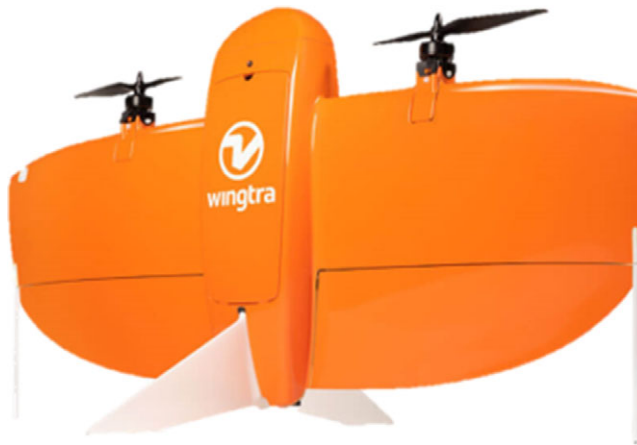
Figure 11. WingtraOne aircraft, a collective thrust transitioning hybrid VTOL UAV. Image adopted from reference [81], with permission.
