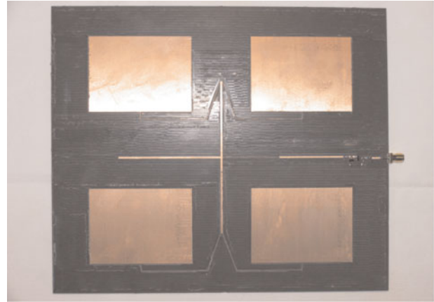
Fig. 5. Photograph of a harvester prototype based on a 2 \times 2 linearly polarized patch antenna array (overall dimensions: 22 \times 19 \text{ cm}^2 ).
