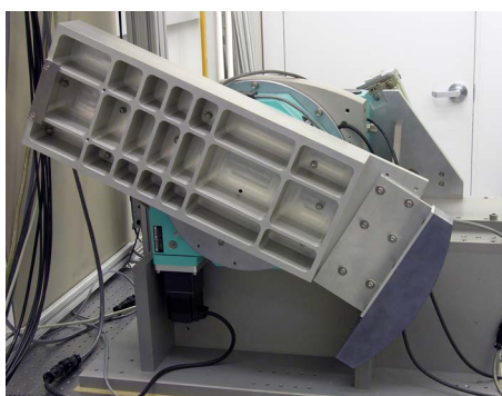
Figure 3. (Color online) Rear view of the CDDBD illustrating stiff and balanced detector arm.
