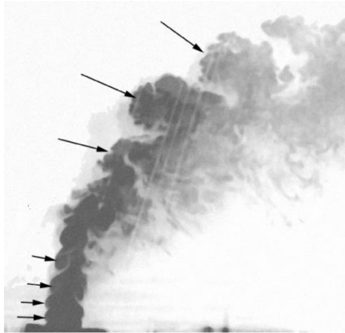
FIGURE 8. Instantaneous visualization obtained by PLIF at the vertical centreplane to illustrate the roll-up process in the upstream jet interface. The arrows indicate the shear layer vortices and how the distance between them is roughly doubled in successive steps.
