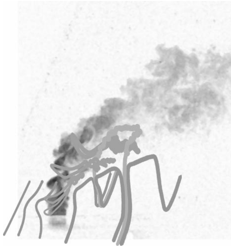
FIGURE 16. Sketch over an instantaneous photograph of the significant vorticity lines and instantaneous structures currently identified in the jet in crossflow. The following are observed: the vortex lines in the wall boundary layer upstream of the jet; the vortex rings as they are folded and wrinkled; the vertical horseshoes from the bottom of the wall to the top of the upper jet interface; and finally the 'handle-type' structures, which are similar to the horseshoes, but located along the lower jet interface, where the cores of the CVP are placed.
