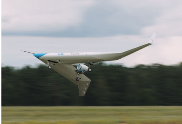
Figure 5. Flight control was experimentally verified using a 5%-scale flight-test demonstrator. Photo: Joep van Oppen for KLM and TU Delft.
