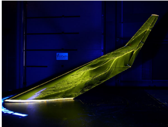
Figure 4. Large vortex structures appear at high angles of attack over the inner wing of the Flying V [11].
