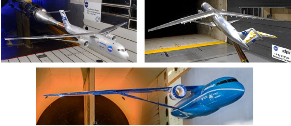
Figure 2. Transonic Truss-Braced Wing high/low-speed and aeroelastic wind tunnel models [6].
