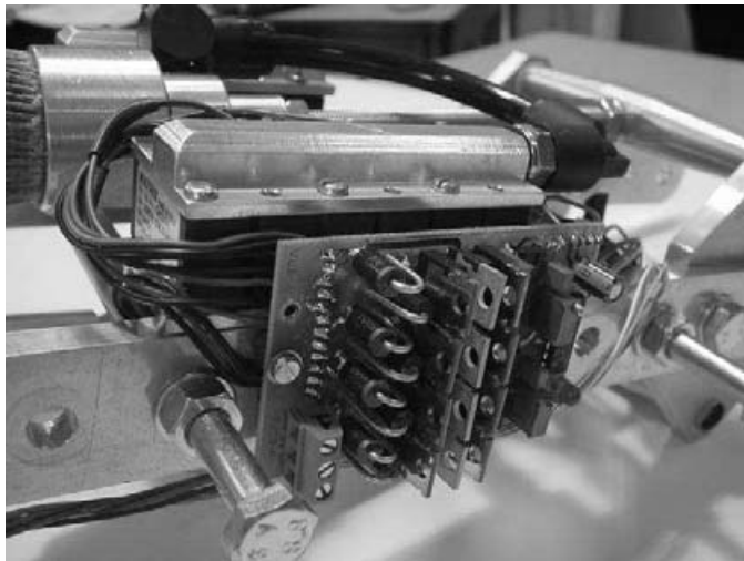
Fig. 7. Detailed view of the valves with speed up circuitry.
