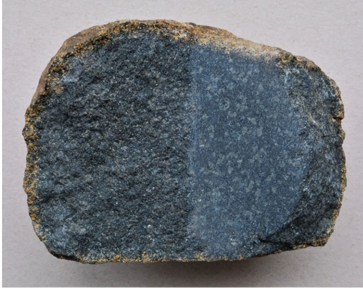
Fig 3. Picrite from the Cwm Mawr Farm quarry, near Hyssington, Powys. A portion of the freshly exposed rock has been ground and polished to demonstrate the appearance of the Church Lawton battle-axe when new and in pristine condition. The length of the rock sample is 120mm, compared to the battle-axe, which is 133mm long. Photograph: Malcolm Reid.
