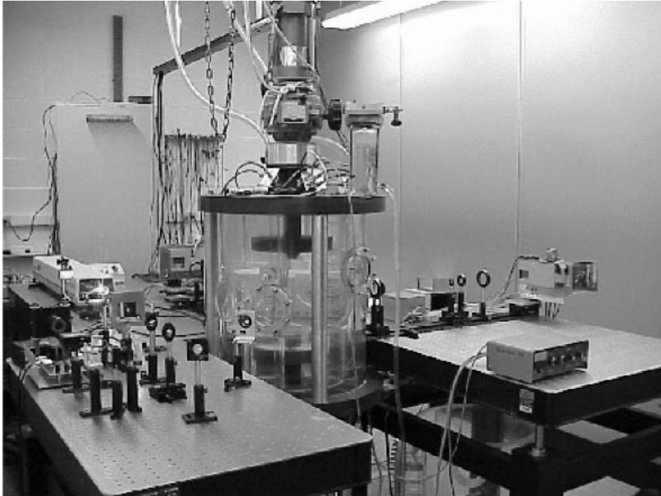
FIGURE 12. Apparatus, consisting of turbulence chamber with counter-rotating disks (foreground), illumination beam entering from foreground and two detectors (background).
