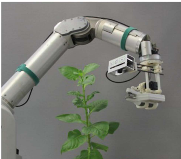
Figure 4. Setup used to take chlorophyll measures from suitable plant leaves, with the Barrett WAM arm carrying a time-of-flight camera and a spad meter. Observe that the leaf-probing task requires clearance (above and below) of a segment in the border of the chosen leaf. (To view this figure in colour please see the online version of this journal.)
