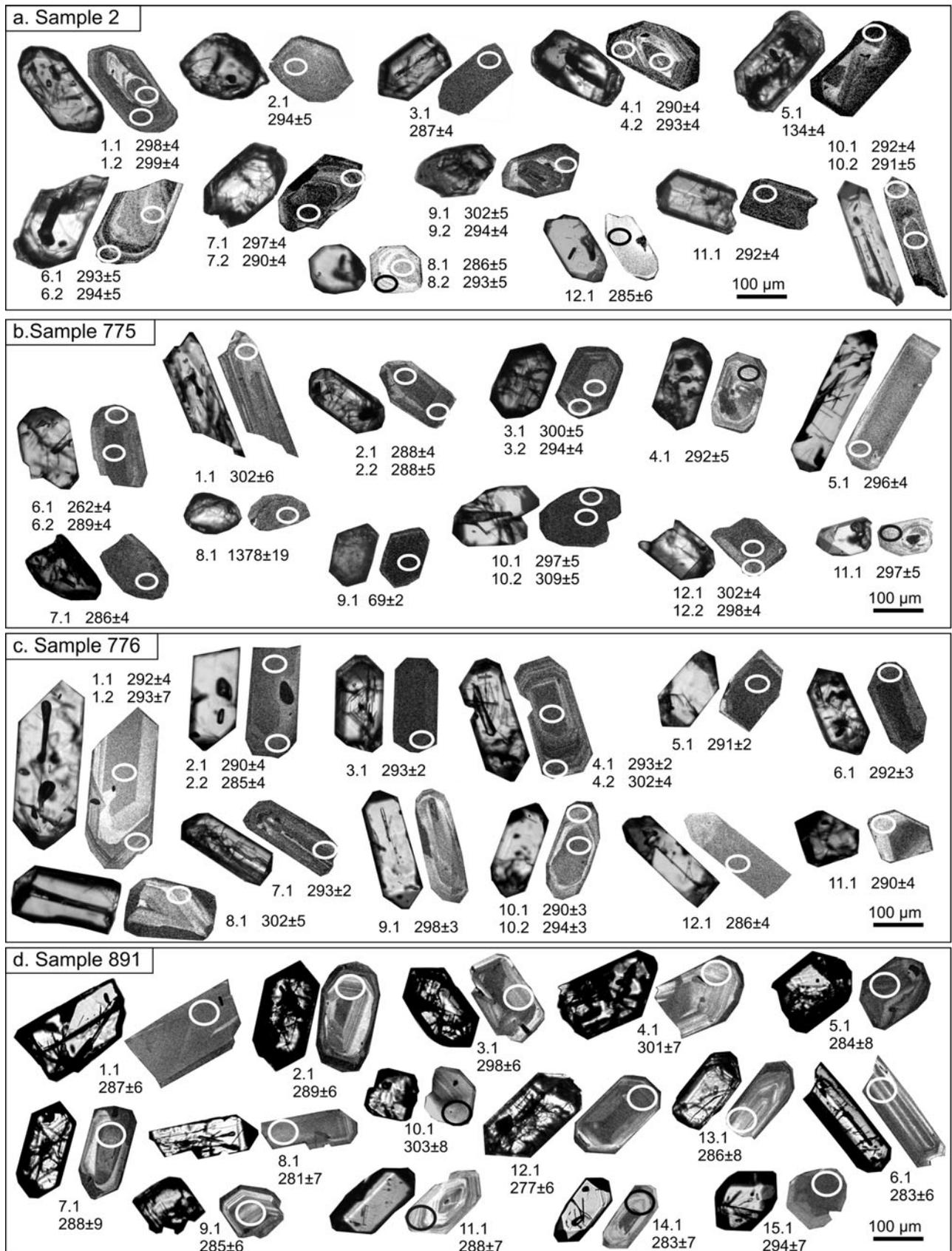
Figure 3. Pairs of optical photomicrographs (left) and cathodoluminescence images (right) of zircons with location of analytical points. (a) Sample 2. (b) Sample 775. (c) Sample 776. (d) Sample 891.  $^{206}\text{Pb}$ – $^{238}\text{U}$  ages and  $1\sigma$  errors are given.
