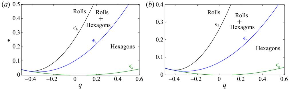
FIGURE 14. Amplitude stability curves in the  $(\epsilon, q)$  plane at  $r = 2.5, Pr = 50$  and two different values of  $\alpha$ : (a)  $\alpha = 0$  Newtonian fluid, (b)  $\alpha = 10^{-4}$  Carreau fluid.
