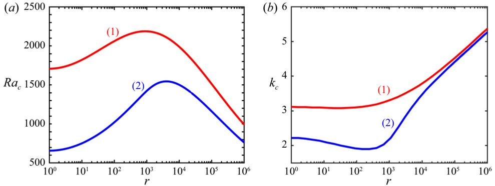
FIGURE 1. Exponential fluid. Critical Rayleigh number (a) and critical wavenumber (b) as a function of the viscosity ratio. (1) NSBC, (2) SFBC.
