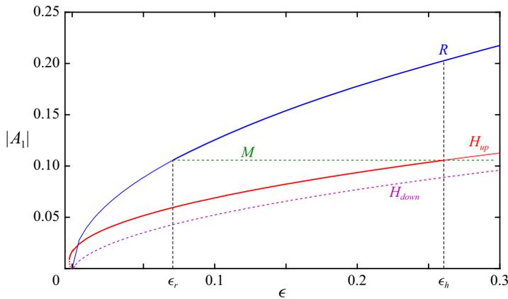
FIGURE 15. Bifurcation diagram for hexagons in the case where  $g_2 > g_1$  with the parameters  $r = 2.5, q = 0$  and  $\alpha = 10^{-4}$ . The amplitude  $|A_1|$  is plotted against the distance to the threshold  $\epsilon$  for the roll-solution branch (labelled  $R$ ), for the mixed mode branch (labelled  $M$ ) and for the two hexagon-solution branches, up- and down-hexagons. Solid lines indicate stable solutions and dashed lines represent unstable solutions.
