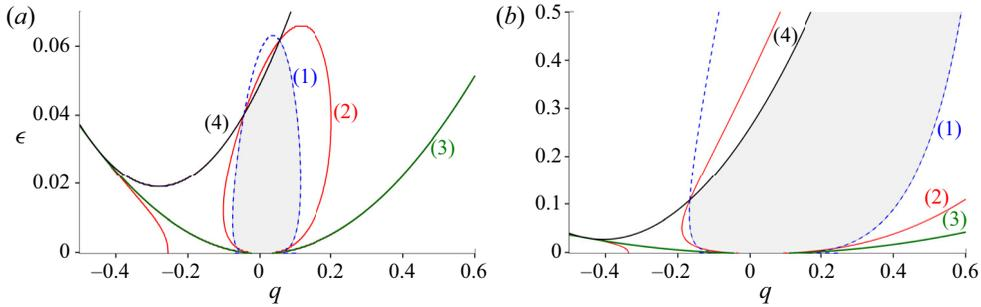
FIGURE 17. Hexagon stability diagram for a Newtonian fluid at  $Pr = 50$  and two different values of the viscosities ratio: (a)  $r = 1.5$  and (b)  $r = 2.5$ . Hexagons are stable inside the grey area. Curve (1):  $D_{\perp} = 0$ , curve (2)  $D_{\parallel} = 0$ , curve (3) bifurcation from the conductive state to convection with hexagons, curve (4) bifurcation from hexagons to rolls.
