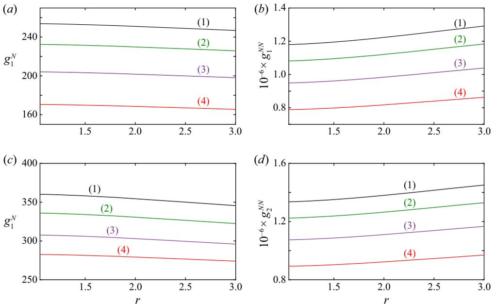
FIGURE 10. (a) ‘Newtonian’ and (b) non-Newtonian contribution to the first Landau coefficient and to the cross-saturation coefficient (c) and (d), respectively, as a function of  $r$  for different values of  $Pr$ . (1)  $Pr = 50$ ; (2)  $Pr = 5$ ; (3)  $Pr = 2$ ; (4)  $Pr = 1$ .
