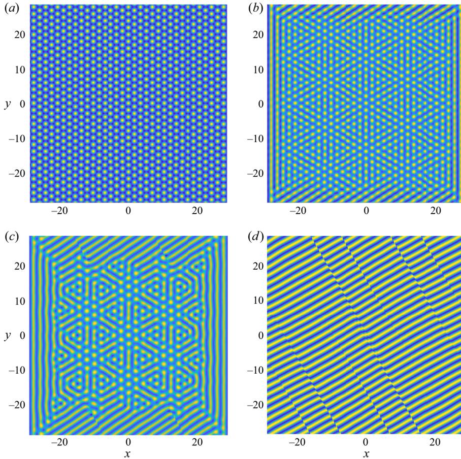
FIGURE 24. Initial condition ( $\mathcal{P}_2$ ): hexagons with  $q = 0.55$ ,  $\epsilon = 0.3$ ,  $r = 2.5$ ,  $\alpha = 10^{-4}$  and  $Pr = 50$ . The reconstructed vertical velocity  $w$  is shown at different times: (a)  $t = 0$ , (b)  $t = 2$ , (c)  $t = 10$  and (d)  $t = 100$ .
