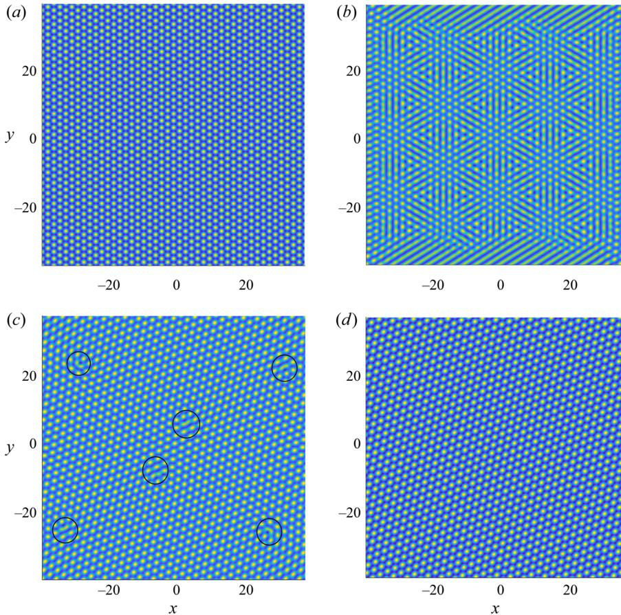
FIGURE 21. Initial condition ( $\mathcal{P}_1$ ): hexagons with  $q = 0.45$ ,  $\epsilon = 0.1$ ,  $r = 2.5$ ,  $\alpha = 10^{-4}$  and  $Pr = 50$ . Contours of the vertical velocity  $w = \sum_{i=1}^3 A_i \exp(i\mathbf{k}_{c,i} \cdot \mathbf{x}) + \text{c.c.}$  for a hexagonal pattern undergoing the transverse instability. The contours are shown at times (a)  $t = 0$ ; (b)  $t = 10$ ; (c)  $t = 1000$  and (d)  $t = 2000$ . In panel (c) the penta-hepta defects are circled.
