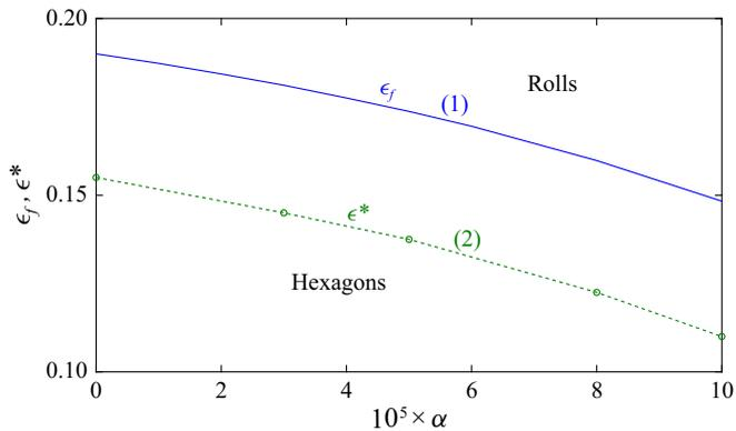
FIGURE 26. Threshold for hexagon–roll transition in the case where there is no distortion of hexagons as a function of the shear-thinning degree, with  $q = 0.55$ ,  $r = 2.5$  and  $Pr = 50$ . (1) Curve of equal energy for hexagons and rolls, (2) numerical simulations.
