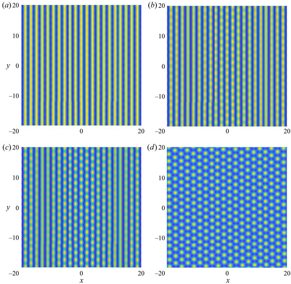
FIGURE 25. Initial condition ( $\mathcal{P}_3$ ): rolls with  $q = 0.25$ ,  $\epsilon = 0.1$ ,  $r = 2.5$ ,  $\alpha = 10^{-4}$  and  $Pr = 50$ . The reconstructed vertical velocity  $w$  is shown at different times: (a)  $t = 0$ , (b)  $t = 11$ , (c)  $t = 15$  and (d)  $t = 2000$ .
