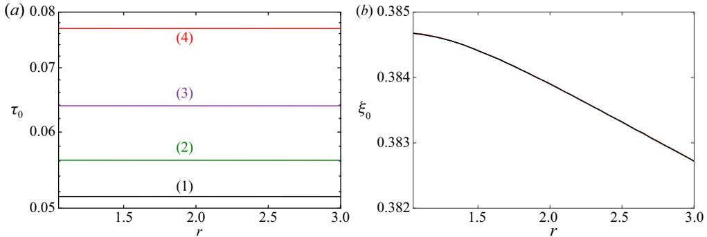
FIGURE 8. Variation of the characteristic time  $\tau_0$  (a) and the coherence length  $\xi_0$  (b) as a function of the viscosity ratio, for different values of Prandtl number. (1)  $Pr = 50$ ; (2)  $Pr = 5$ ; (3)  $Pr = 2$ ; (4)  $Pr = 1$ .
