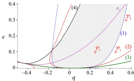
FIGURE 20. Hexagon stability diagram for a shear-thinning fluid with  $\alpha = 10^{-4}$ ,  $Pr = 50$  and  $r = 2.5$ . The curve  $\epsilon_r(q)$  is a boundary above which rolls are stable with respect to homogeneous perturbations. (+) Points where numerical simulations were performed.
