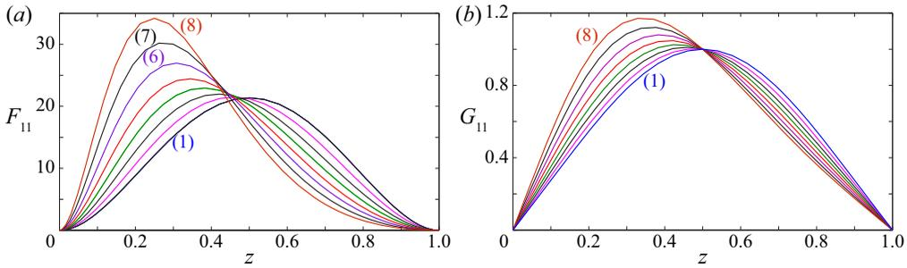
FIGURE 2. Exponential fluid. (a) Vertical velocity eigenfunction and (b) temperature perturbation at the first order as a function of the depth  $z$  for different values of the thermodependency coefficient  $c$ . (1)  $c = 0$ ; (2)  $c = 1$ ; (3)  $c = 2$ ; (4)  $c = 3 \dots$  increasing  $c$  by step 1 until curve (8)  $c = 7$ .
