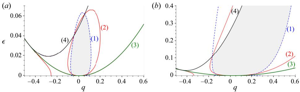
FIGURE 18. Hexagon stability diagram for a shear-thinning fluid with  $\alpha = 10^{-4}$  at  $Pr = 50$  and two different values of the viscosities ratio: (a)  $r = 1.5$  and (b)  $r = 2.5$ . Hexagons are stable inside the grey area.
