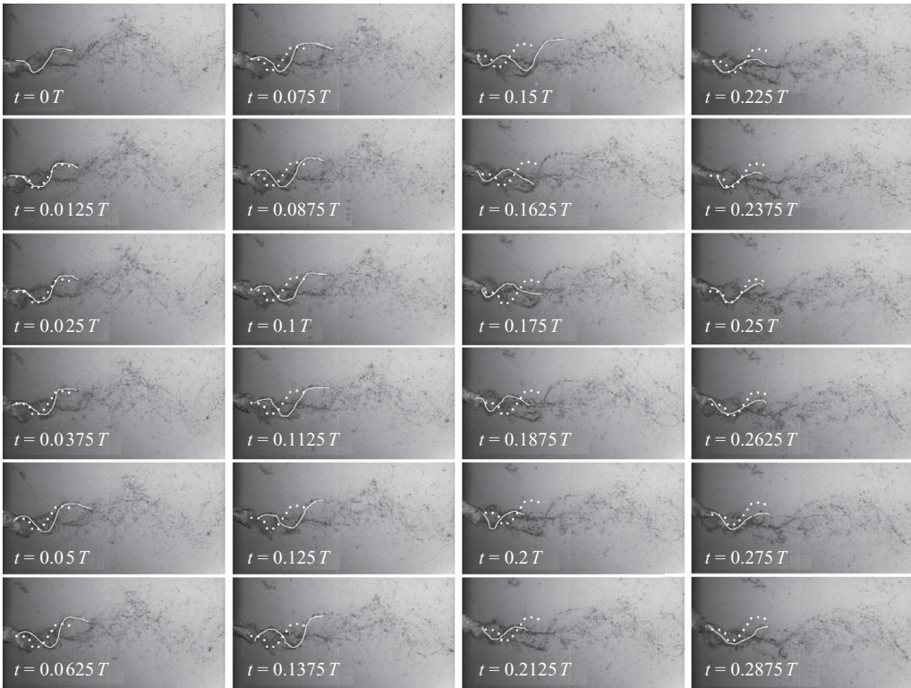
FIGURE 26. Double-helix breakdown for the four-bladed propeller. Dotted lines represent the cavitating traces of the reference filament of the double helix at t = 0 , and solid lines represent the current cavitating traces of the reference filament of the double helix. The best alignment between dotted and solid lines appears after about \Delta t = T/4 .
