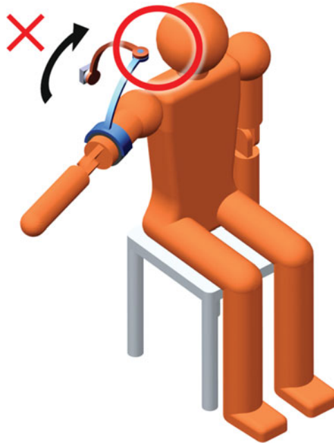
Fig. 3. (Colour online) A 3R exoskeleton with the base joint behind the shoulder cannot raise the upper arm above the horizontal plane as this will cause the mechanism to collide with user's head.
