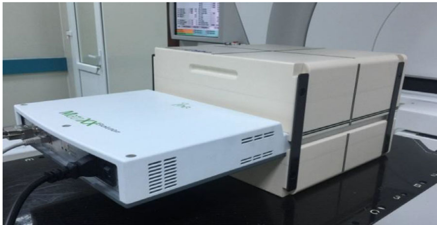
Figure 1. MatriXX Evolution and MULTICube Phantom.
