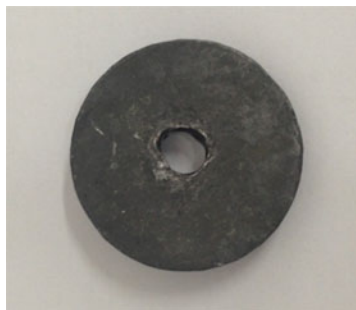
Fig. 12. Lead plate ripped through by HNS-IV with the charge density of 1.6 g/cm 3 .
