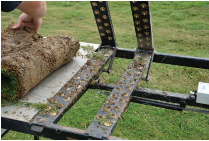
Figure 1. Apparatus used to measure hybrid bermudagrass ( C. dactylon × C. transvaalensis Burt-Davy, cv. ‘Tifway’) sod tensile strength at harvest during (377 d after sprigging) during field experiments conducted in Knoxville, TN during 2010 to 2011 and 2012 to 2013.
