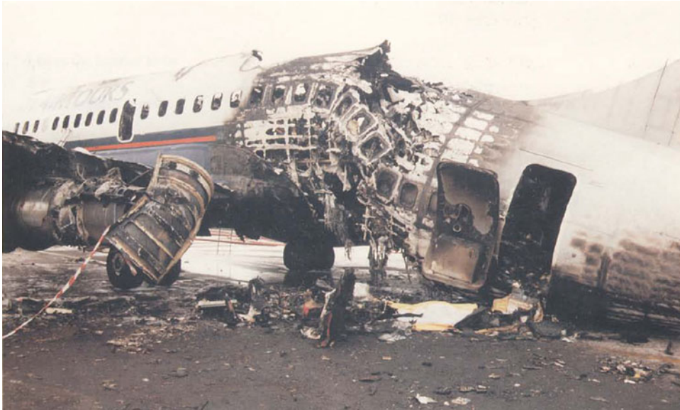
Figure 1. (Colour online) Damage to the B737-236 fuselage in the Manchester accident (1) .
