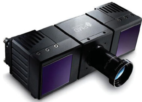
Fig. 8. PMD CamCube consisting of camera and illumination unit.
