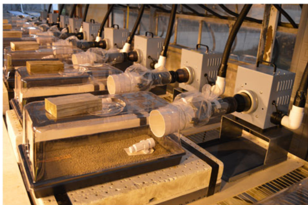
Figure 1. Humidome setup for research showing soil in tray, HOBO temperature, and relative humidity sensor, sampling connections, and air sampler.
