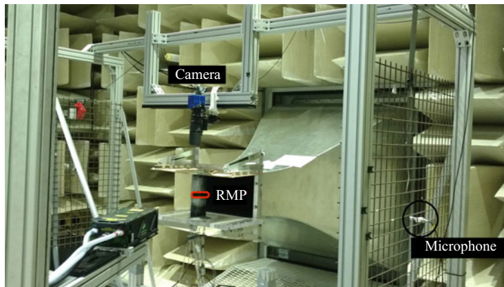
Figure 3. Planar PIV set-up for synchronised velocity–pressure measurements.
