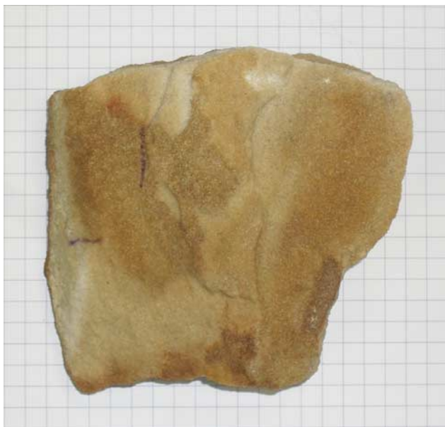
Fig. 1. Image of Beacon Sandstone sample used in this study, from Linnaeus Terrace, Upper Wright Valley, Antarctica. Background grid is 0.5 cm squares.
