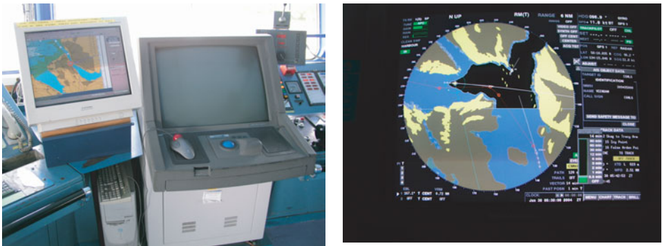
Figure 5. A variation on a theme. The ECDIS PPI on the right is correctly set-up to identify any datum discrepancies between the chart and the ground stabilisation of the radar display. A low-cost, but effective alternative is the chart display situated adjacent to the ARPA as fitted on the 30 year old passenger ferry Stena Europe. Separate equipments facilitate the comparison of information which is critical to safe navigation.
