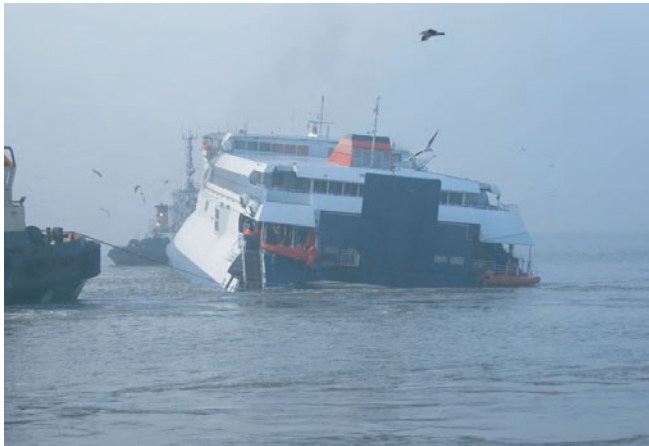
Figure 2. The Sea Express 1 is towed to safety after the collision on the River Mersey. Poor bridge team management was cited as a reason for the collision, however, it was arguably the fact that the Sea Express 1 continued her intended track irrespective of the thick fog, thereby getting so close to the Alaskan Rainbow that avoiding action could not be taken (Courtesy of MAIB).
