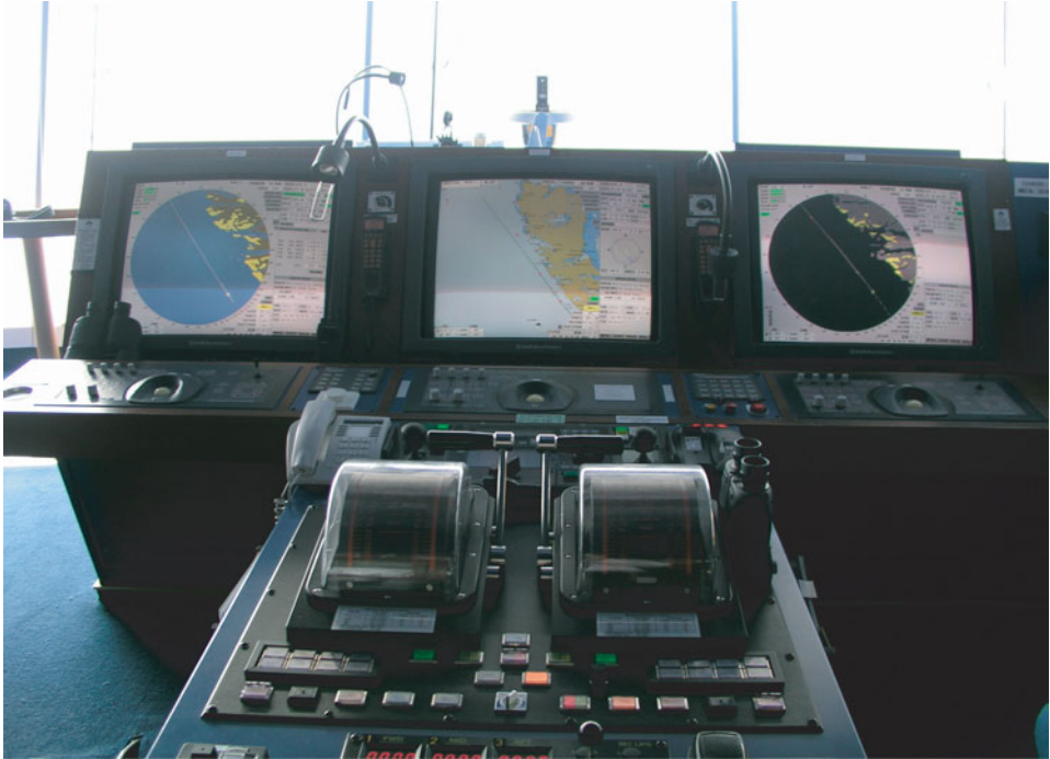
Figure 4. The ATLAS NACOS integrated bridge system.
