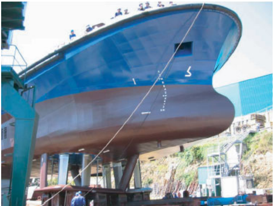
Figure 11. Photo showing the escort tractor Voith tug "VELOX" moments before the launching at the Spanish shipyard, Gondán S.A. on 03.07.04. This tug is the first of this type in the world that incorporates a bulbous bow. Photo: author.
