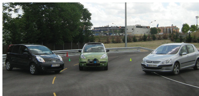
Fig. 1. (Colour online) Test vehicle with radars mounted on the bumper (center), black colored car (left) and gray (silver) colored car (right).
