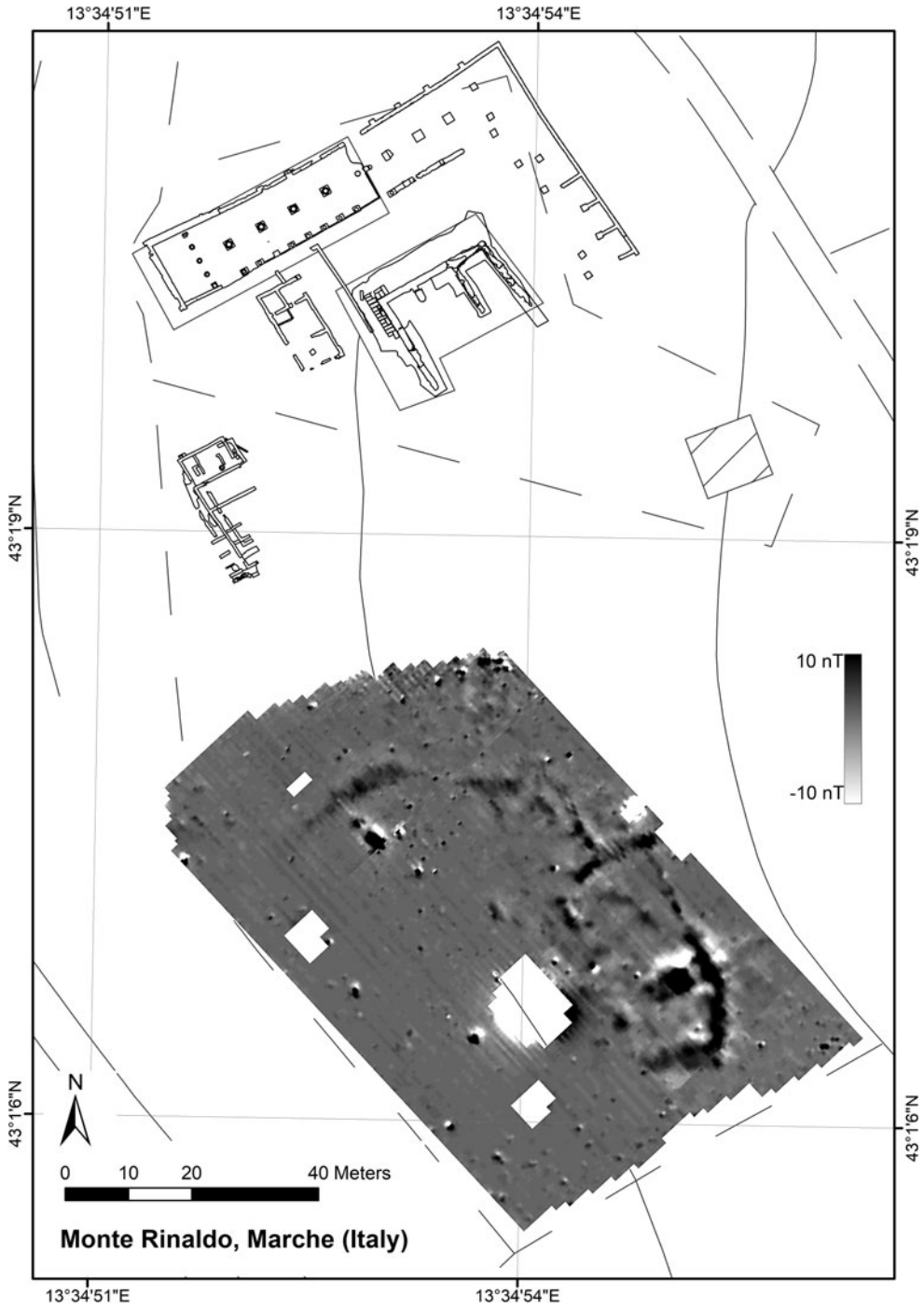
Fig. 2. Results of the magnetometer survey at Monte Rinaldo (Image E. Pomar).
