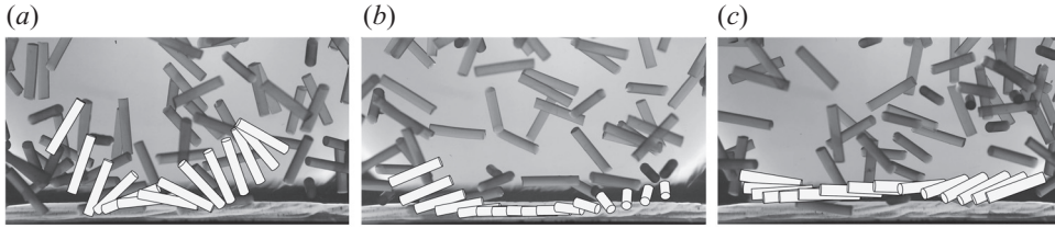
Figure 4. Three typical examples of how particles of length 2.5 cm and diameter 0.45 cm interact with bottom BL at Ra \approx 2.1 \times 10^9 . Successive snapshots (white cylinders) showing particles moving from left to right, as extracted from a video with a time interval of 1.0 s for (a,c) and 0.7 s for (b). The background pictures are taken from the last frame. (a) A particle briefly collides twice with the BL and returns to the bulk. (b) A particle slides along the BL. (c) A particle hovers above the BL.
