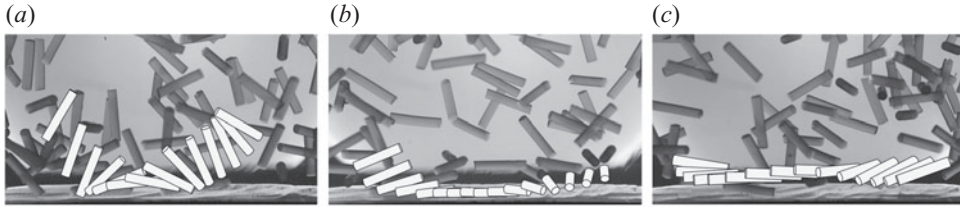
Figure 4. Three typical examples of how particles of length 2.5 cm and diameter 0.45 cm interact with bottom BL at Ra \approx 2.1 \times 10^9 . Successive snapshots (white cylinders) showing particles moving from left to right, as extracted from a video with a time interval of 1.0 s for (a,c) and 0.7 s for (b). The background pictures are taken from the last frame. (a) A particle briefly collides twice with the BL and returns to the bulk. (b) A particle slides along the BL. (c) A particle hovers above the BL.
