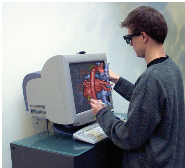
Figure 4. Stereoscopic glasses bring the virtual model “out of the screen” to obtain a full three-dimensional understanding. Styluses track the position and orientation of each hand, shown with yellow jacks in the model, and provide input for a gesture-based interaction interface.
