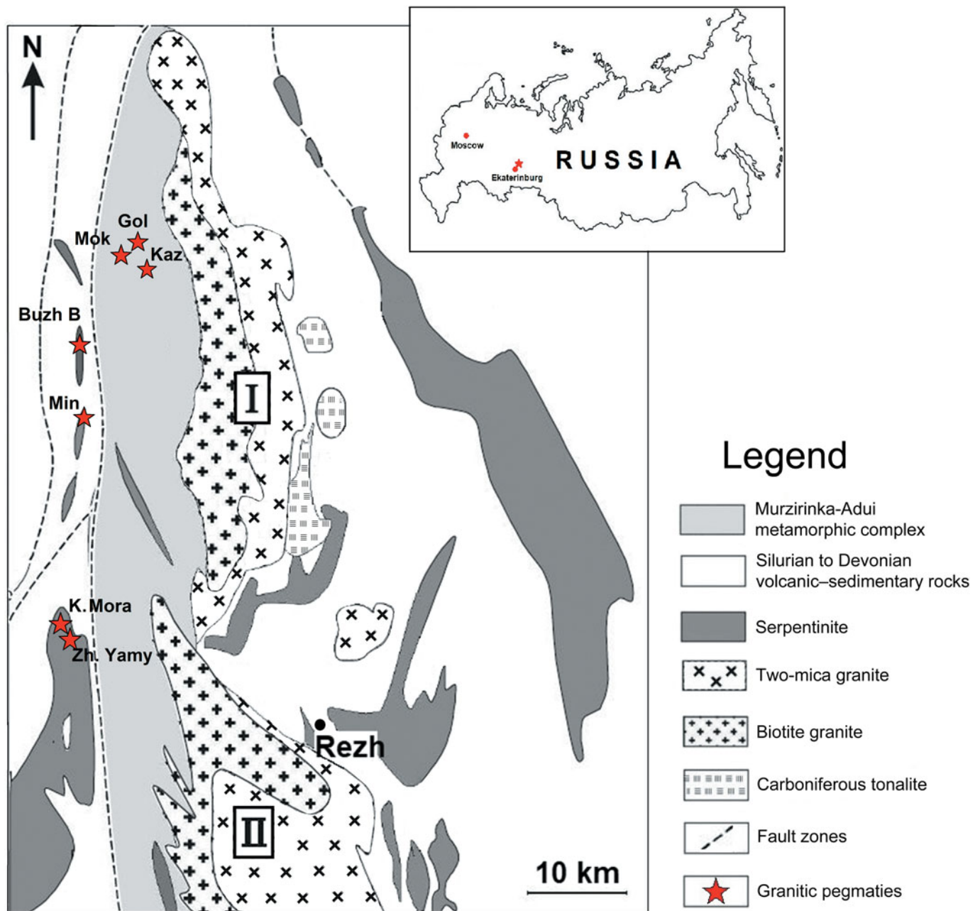
Fig. 1. Geological sketch map of Murzinka granite pluton (I), modified after Fershtater and Borodina (2018) and (II) Adui granite pluton. Pegmatites: Mokrusha (Mok); Golodnaya (Gol); Kazennitsa (Kaz); Buzheninov Bor (Buzh B); Ministerskaya (Min); Kopi Mora (K. Mora); and Zheltyye Yamy (Zh. Yamy). The Geographical location of the area studied is marked with a star in the inset.
