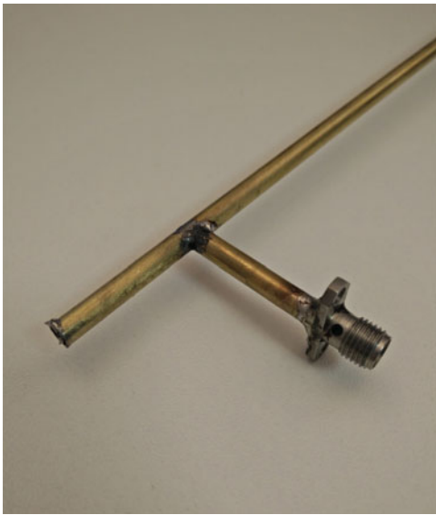
Fig. 2. Initial prototype utilizing 90° microwave feed.
