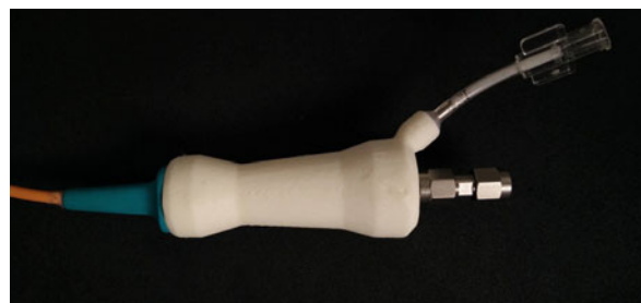
Fig. 8. Photograph showing the final 3D-printed handpiece design.
